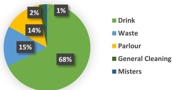
**Figure 1.** Breakdown of total water use (%) including drinking, waste (water not recovered from plate cooler return and pasture bowl spillage), parlour (foot baths, parlour floor cleaning, cow cleaning, line sanitization), general cleaning (barn floor, farm equipment), and mister water use.
